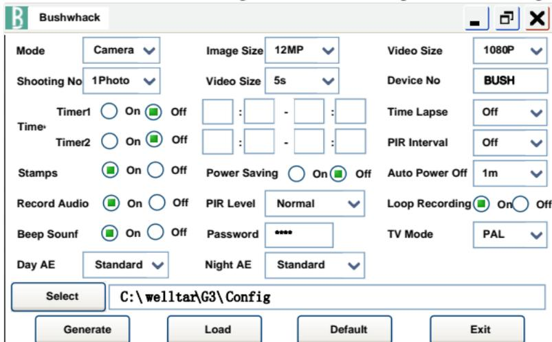
After parameter setting, click on the "Select" to select the file storage address. Click "generate" to generate the camera parameter settings file. Click "Exit" to exit the main menu interface.
